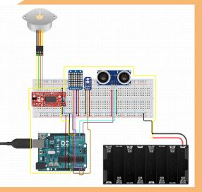
The figure on the right is representative of how all the components will fit together from a wiring perspective
